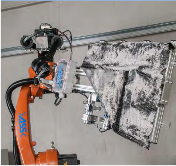
Handling of CFRP
