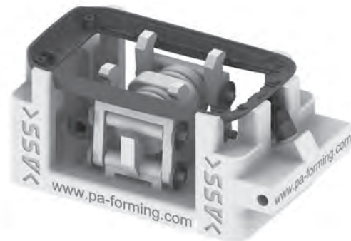
Special gripper with integrated movable functions for mobile phones
